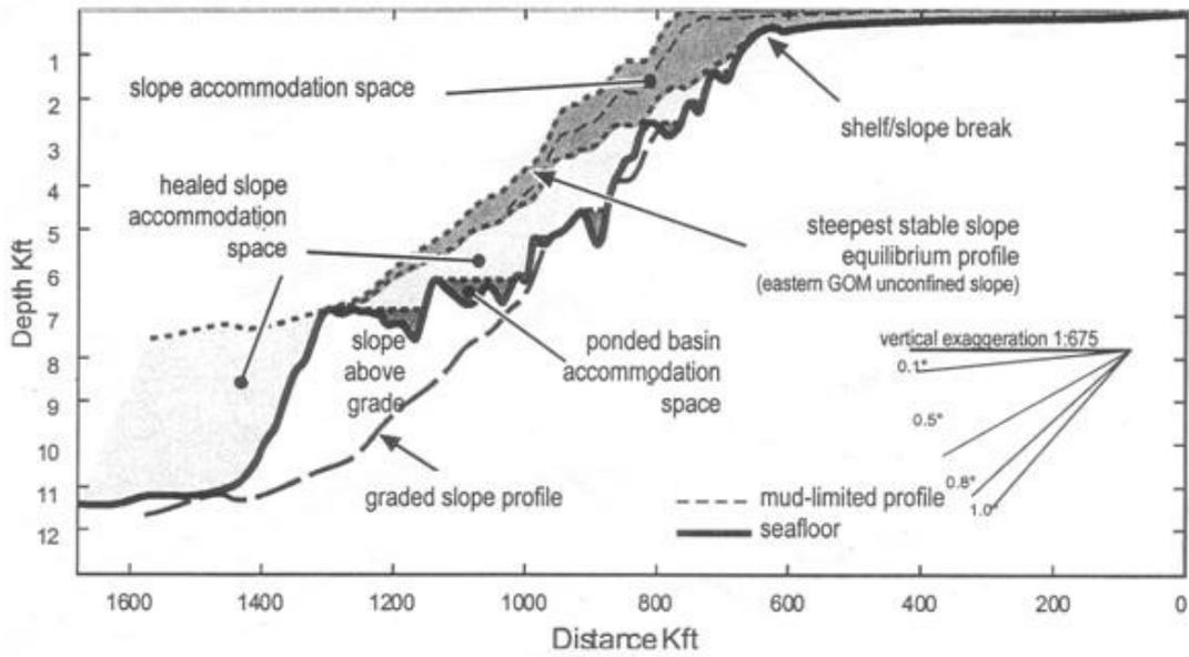
Figure 8 Accommodation spaces for sediments developing on the slope profile (Prather, 2001).
