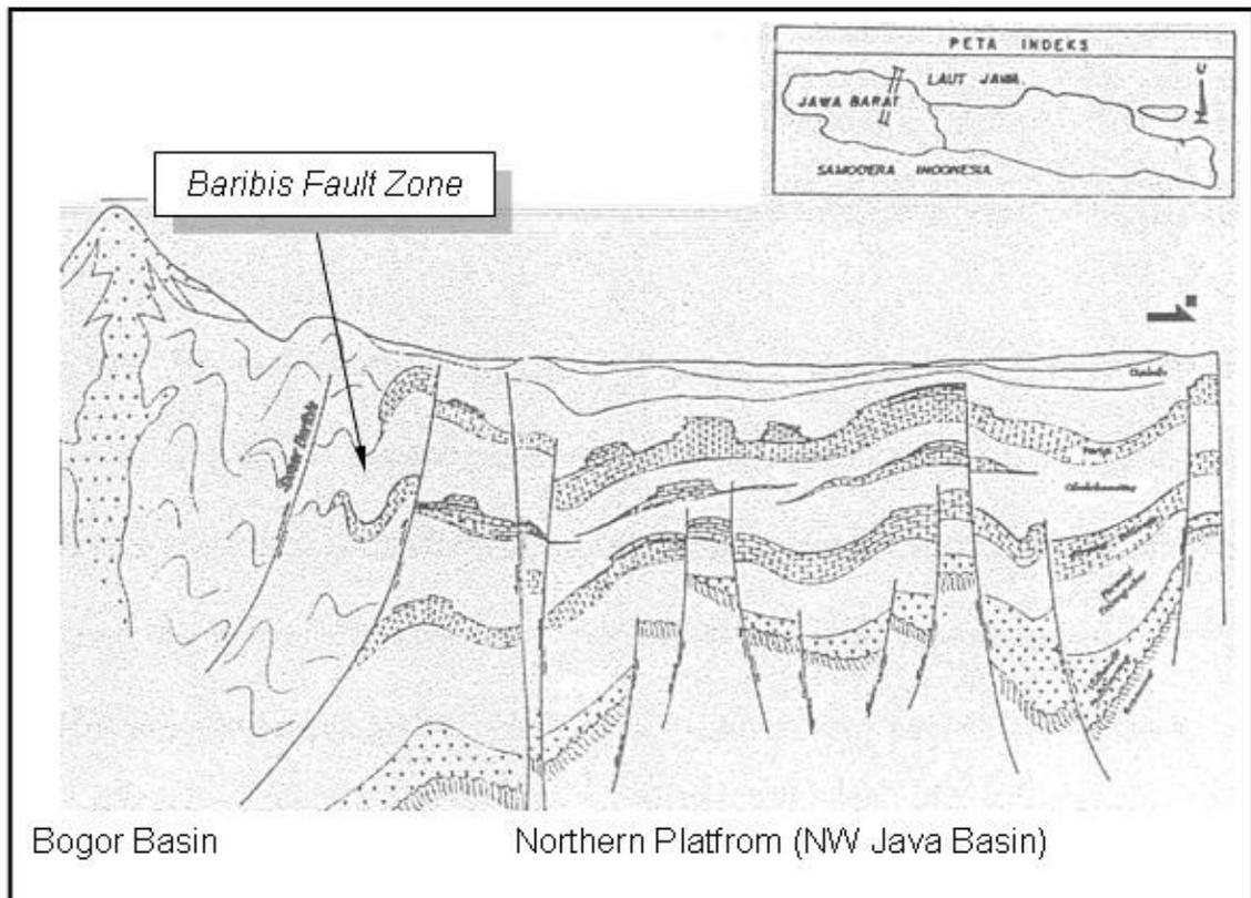
Figure 5 Inverted Baribis Fault positioned on the margin between the Northern Platform and the Bogor Basin (Supriyanto and Ibrahim, 1993)
