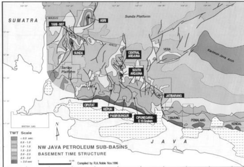
Figure 6 Basement time structure map of NW Java Basin showing petroleum sub-basins (Noble *et al.*, 1997)
