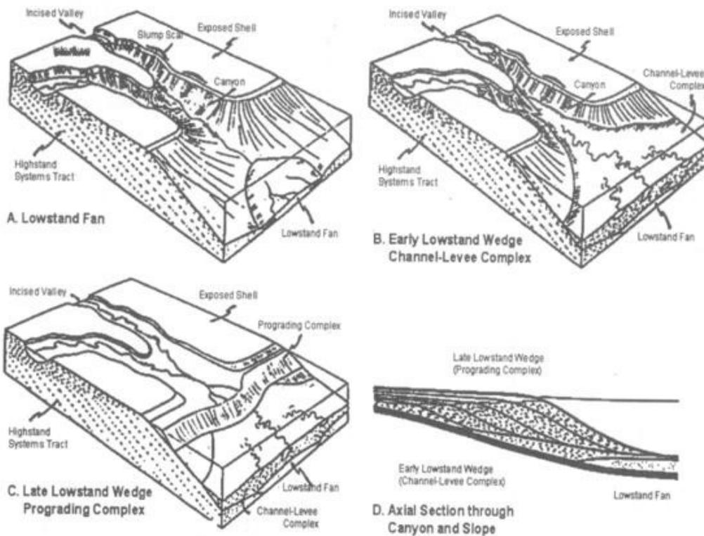
Figure 9 Models for sub-marine fan deposition (Posamentier *et al.*, 1991 in Nugrahanto *et al.*, 2001).
