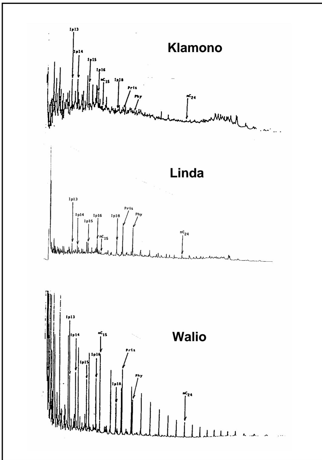
Figure 4 C10+ saturated GC scan of Klamono and Linda oils (biodegraded) and Walio oil (non-biodegraded)
