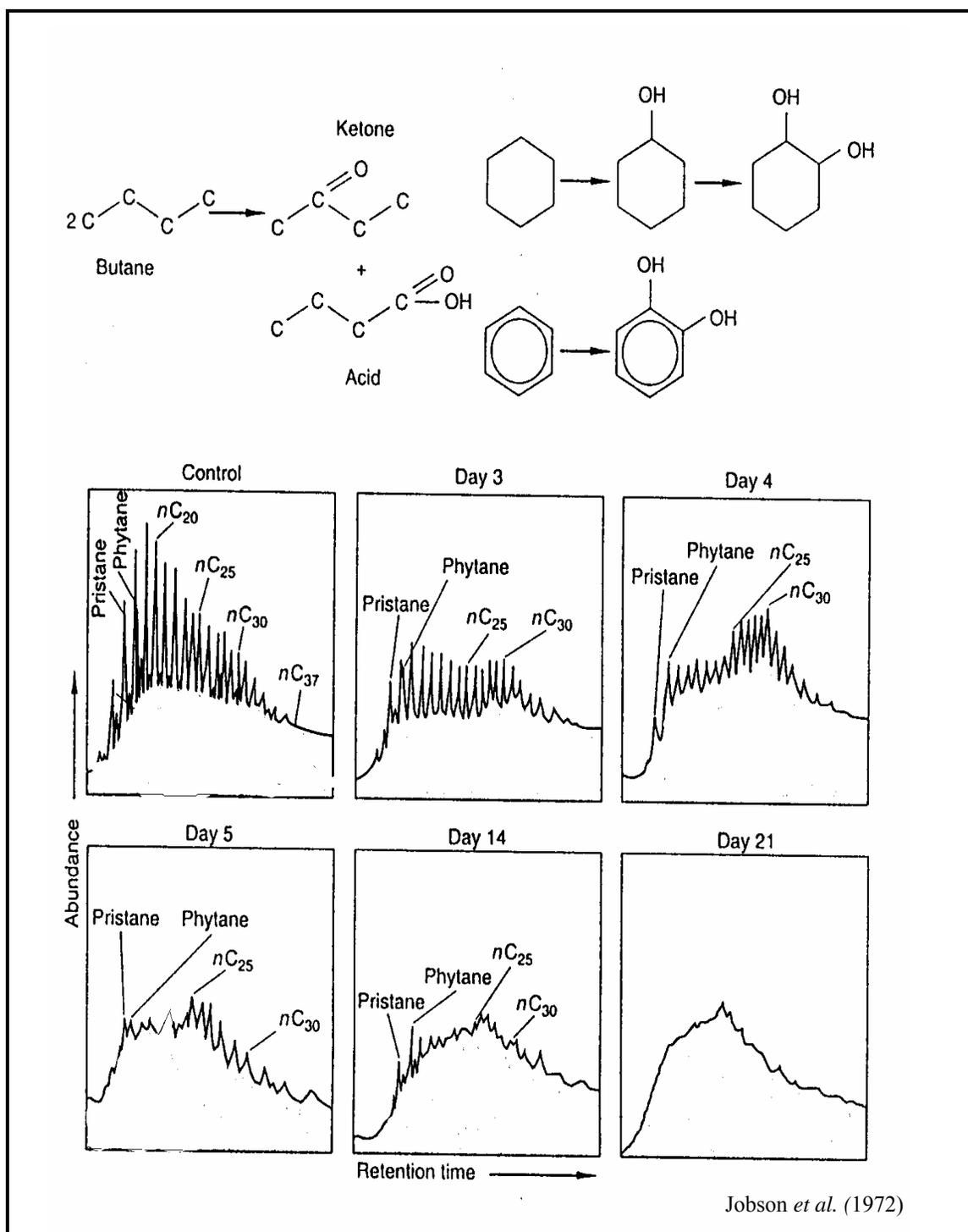
Figure 1 Biodegradation is oxidation of hydrocarbons to result in ketones, acids, and alcohols. Treatment of bacteria culture on Saskatchewan oil cause sequential disappearance of  $n$ -paraffins in 21 days of incubation.
