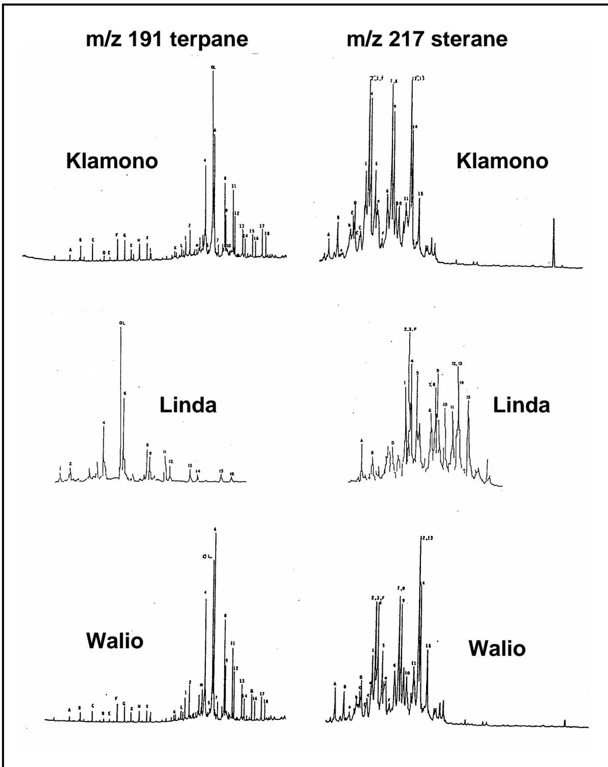
Figure 5 GC/MS scan m/z 191 (terpane) and m/z 217 (sterane) of Klamono, Linda, and Walio oils showing similar distribution indicating no attack of biodegradation on terpane and sterane of Klamono and Linda oils.
