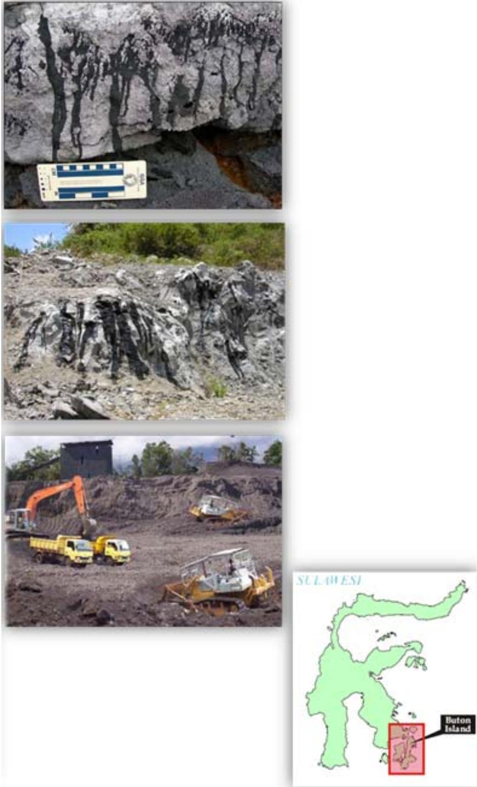
**Figure 4b** - Some photographs showing asphaltic rocks at Buton Island as impregnated materials/bitumen of the rocks. The rocks are 15-35 % impregnated by asphalt/bitumen. Lowermost photograph shows mining work of asphalt deposits at Buton Island.
