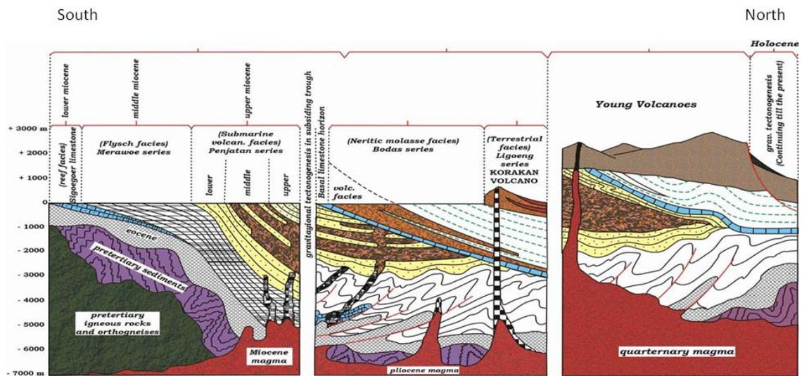
**Figure 8** - Schematic section across Central Java showing uplift of the South Serayu Range (south) and subsidence of North Serayu (north). Thick sediments were deposited into North Serayu and deformed by gravity tectonics tectonics as thin-skinned fold and thrust belts. The structures were then covered by thick volcanic-clastic deposits of Late Neogene into Pleistocene (van Bemmelen, 1949; Satyana and Armandita, 2004).
