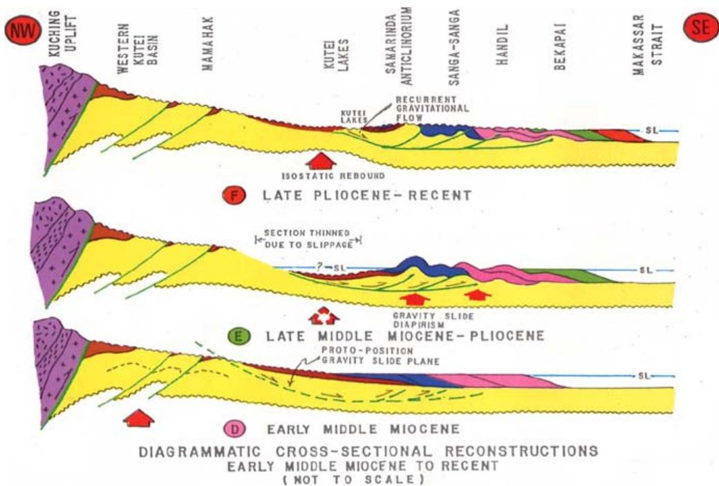
**Figure 5** - Upper Kutei Basin, East Kalimantan showing Samarinda Anticlinorium as principal structural elements in the eastern Kutei Basin (Ott, 1987). Lower. Schematic sections (location of section see map of Kutei Basin) showing the evolution of Samarinda Anticlinorium formation by gravity tectonics (Ott, 1987).
