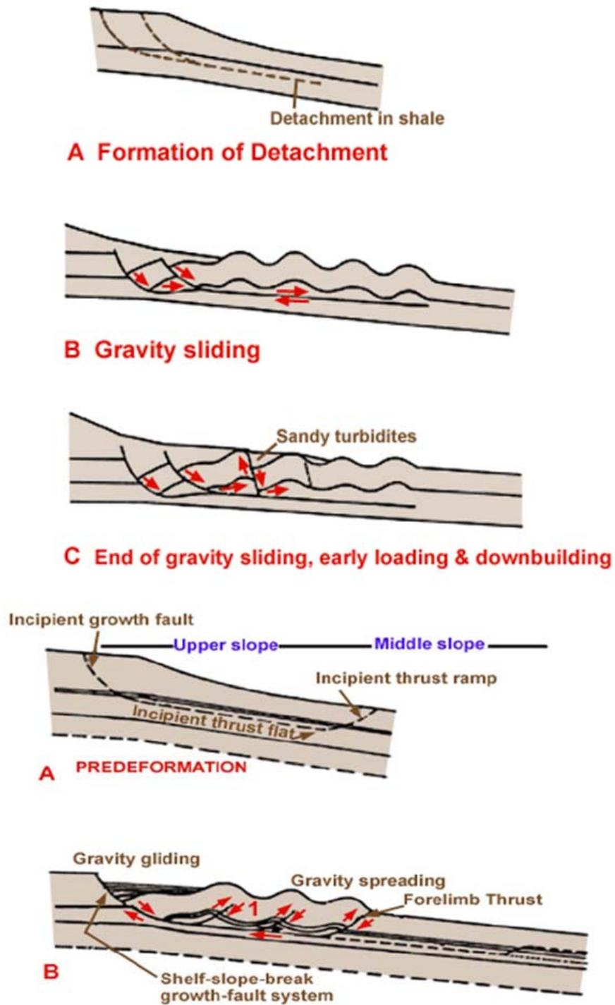
**Figure 1** - Stages of gravity tectonics/ gliding tectonics/gravity sliding, including a formation of detachment/decollement surfaces and formation of thin-skinned fold and thrust belts by gravity sliding. (<http://oilandgastraining.net>).
