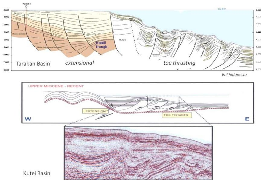
**Figure 6** - Gravity tectonics in offshore Tarakan and Kutei Basins, represented by Samarinda Anticlinorium and toe thrusting in Kutei Basin and growth faults as well as toe thrusting in offshore Tarakan Basin.
