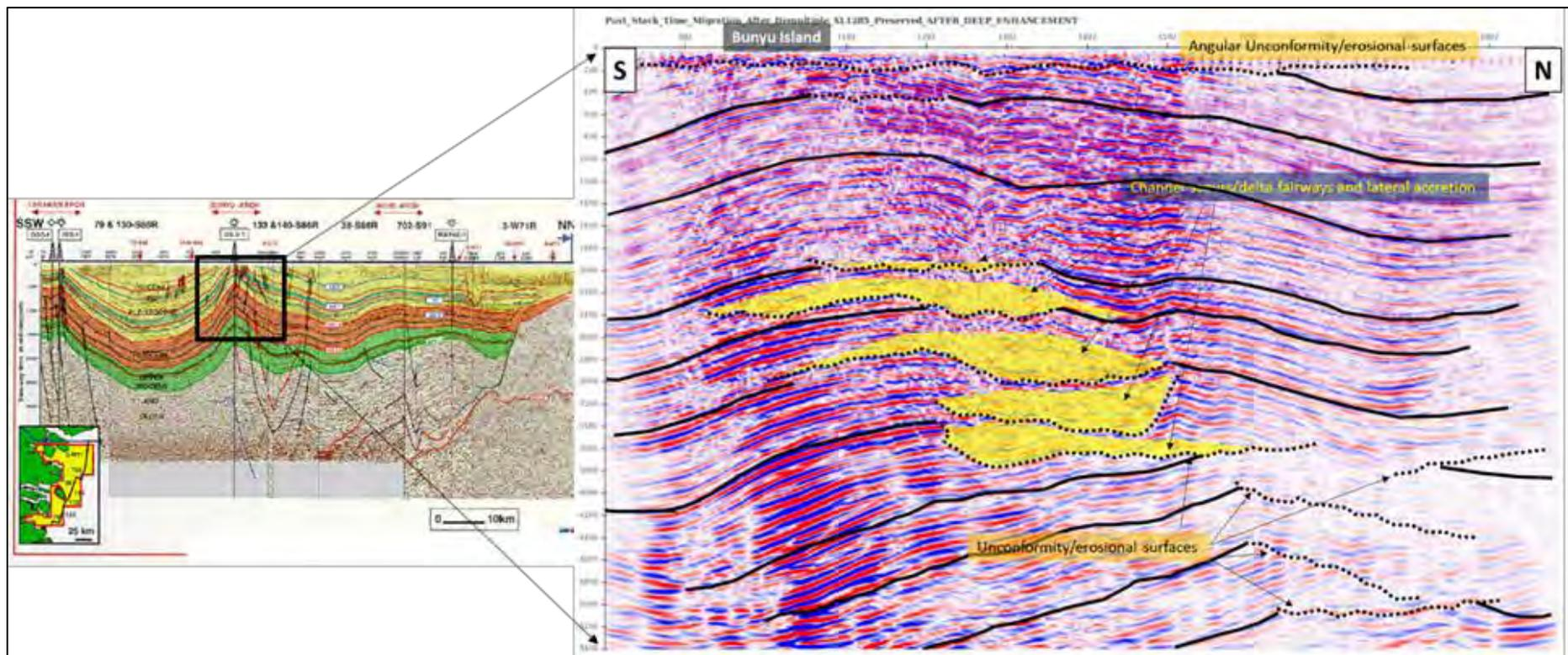
**Figure 6** - Eroded Bunyu Arch as accommodation areas for the upcoming delta sedimentation.
