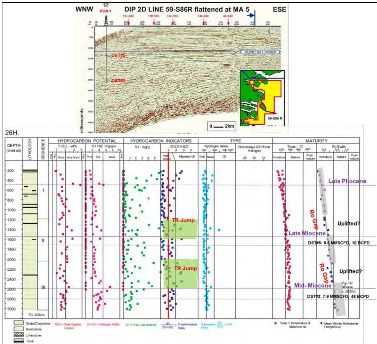
**Figure 8** - Stratigraphic trap: hydrocarbon accumulation before structure development in Bunyu flank. Seismic section flattened show that gas accumulated before structural development (from Sebangang I PSC report of Total, 2000).
