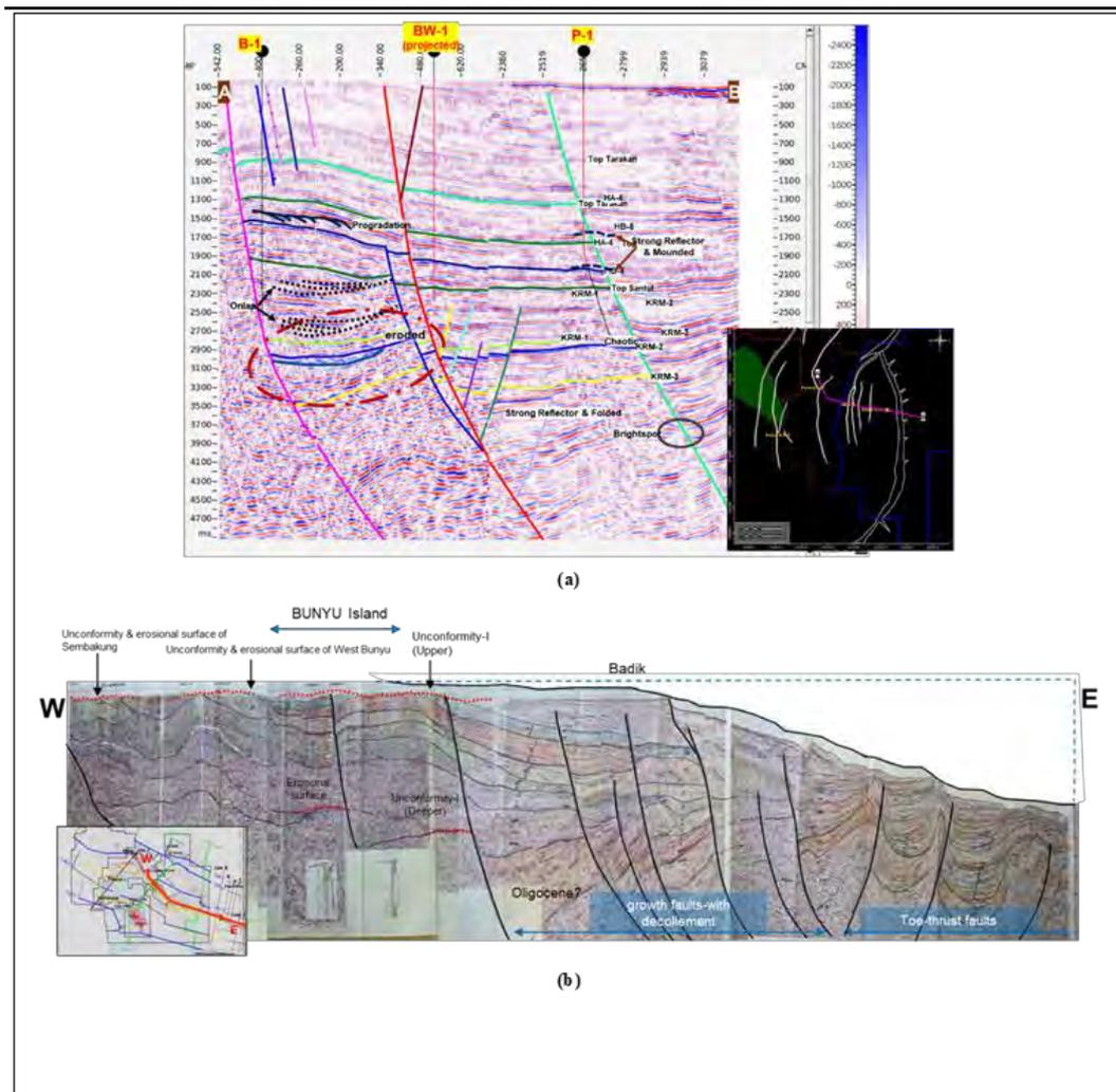
**Figure 7** - Unconformity I located in Bunyu area, shows erosional and angular unconformity surface created by reactivated listric normal fault. (a) Erosional surface at Deeper zone (b) uplifted island and truncated surfaces of Bunyu.
