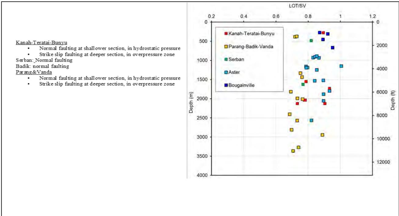
**Figure 4 -** Composite Leak of Test (LoT) versus vertical stress (Sv) plot. Source: Pore Pressure PHENC.
