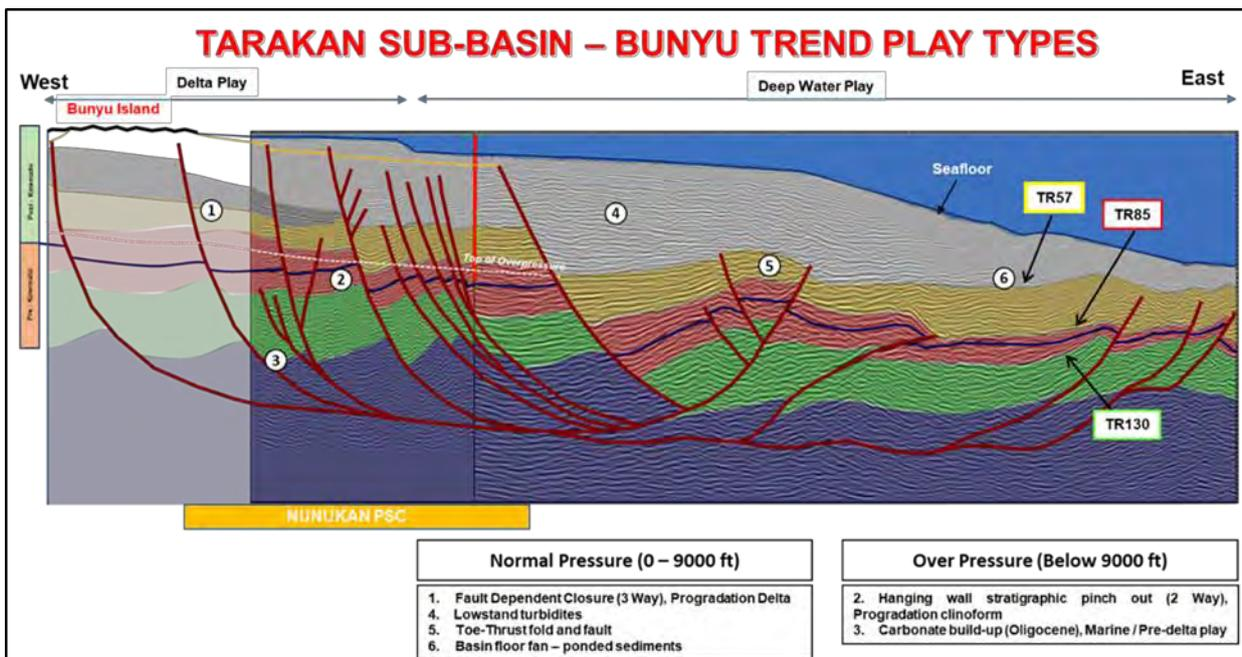
**Figure 10** - Tarakan Sub basin Bunyu Trend Play Types, classified by subsurface pressure zone.
