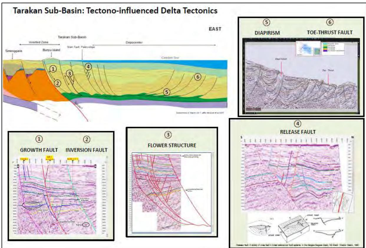
**Figure 3** - Tarakan Sub basin as Miocene to Pleistocene Tectono-influenced Delta Tectonic element: Growth fault, Inversion, Flower structure, Release fault, Diapirism and Toe Thrust fault.
