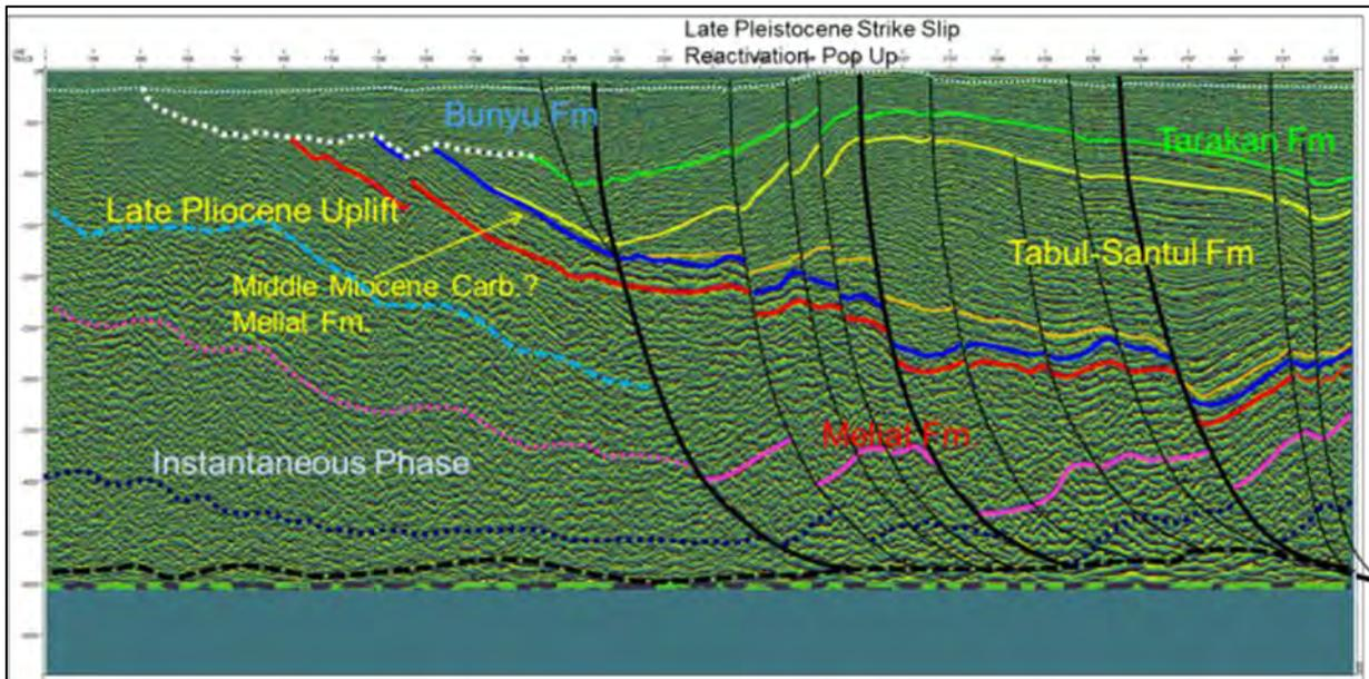
**Figure 9** - Unconformity II surface with significant erosional/truncated surface indicates intensive compressional stress during Pliocene to Pleistocene.
