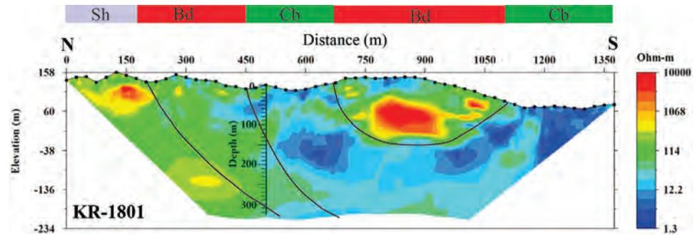
**FIGURE 8** Resistivity model of KR18-02 (Dakah). The color bar on the top indicates the geological outcrop (Cb, clay breccia; Bd, basalt and diabase; Vb, volcanic breccia). The basalt-diabase bodies at the surface are distributed in some distances. But there is one relatively larger high resistivity body to the depth of 100 meter
