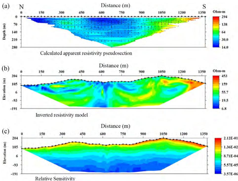
**FIGURE 6** Resistivity result of KR18-03 (Wagirsambeng). From top to bottom: (a) Calculated apparent resistivity pseudosection. The black dots indicate datums used in inversion modeling. (b) Inverted resistivity model, which indicates small variation of the resistivity values (the highest only about 450 ohm m). (c) Relative sensitivity section. The sensitivity distribution is almost normal in all part of section, where the value is decreasing to the depth
