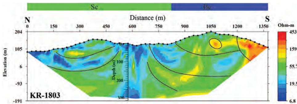
**FIGURE 9** Resistivity model of KR18-03 (Wagirsambeng). The color bar on the top indicates the geological outcrop (Sc, scaly clay; Bc, basalt and cherts). The high resistive bodies in this section represent the basalt-cherts, which has about 100 m thickness at the south edge of the section
