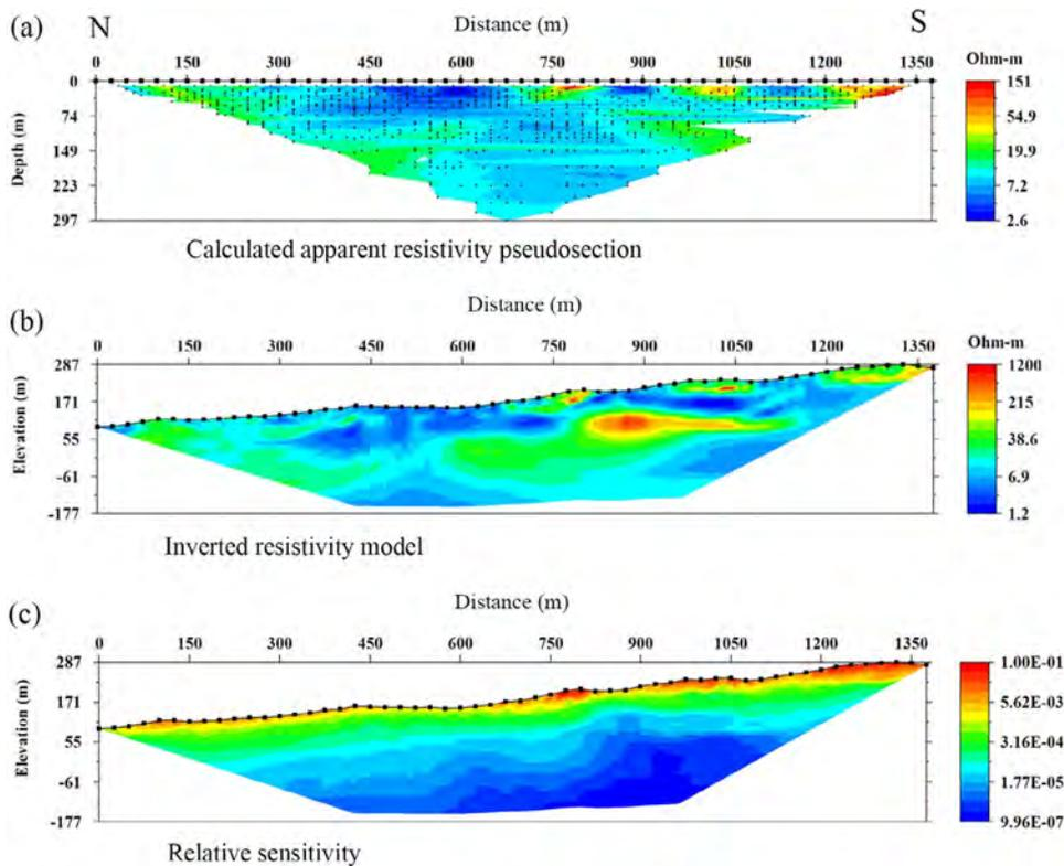
**FIGURE 5** Resistivity result of KR18-02 (Dakah). From top to bottom: (a) Calculated apparent resistivity pseudosection. The black dots indicate datums used in inversion modeling. (b) Inverted resistivity model. There are only few small bodies of high resistivity, with the highest resistivity only about 1200 ohm m. (c). Relative sensitivity section. The sensitivity discontinuity is at about the large area of relatively higher resistivity cluster
