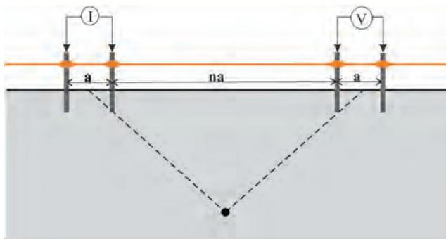
**FIGURE 3** Sketch of electrodes configurations ( $a$  is the distance between two electrodes,  $na$  is the total distance of  $n$  electrodes). We used 56 electrodes with  $a = 25$  m at each line of measurement
